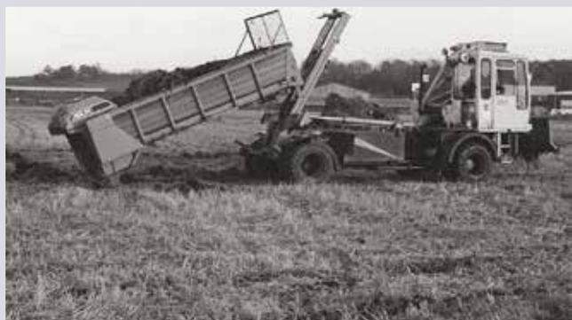
*Specially adapted manure spreader demonstrating the hook lift-type load-carrying system on the NIAE transport tractor © Supplied by Mike Williams*
