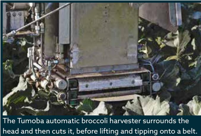
The Tumoba automatic broccoli harvester surrounds the head and then cuts it, before lifting and tipping onto a belt.
